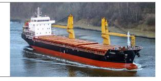
NKK **CLASS SUEZ CANAL (NET)** 5506.31 PANAMA CANAL (NET) 5635 IMDG / IMSBC / GRAIN FITTED? Yes / Yes / Yes MAIN ENGINE Daihatsu 8DKM-28, 2500 kW, 750 rpm **AUXILIARY ENGINE** 3 x MWM HND with each 273 kW **CARGO GEAR** 2 cranes, SWL 45 mt - combination up to 90 mt, situated portside, one spreader o/b, max slewing radius: 22 m (at 25 deg), min slewing radius 4.50 m, hoisting speed: 45 mt 7 m/min - 27 mt - 10.5 m/ min - 9 mt - 21 m/min, luffing time 56s, slewing speed: 0.35 rpm
